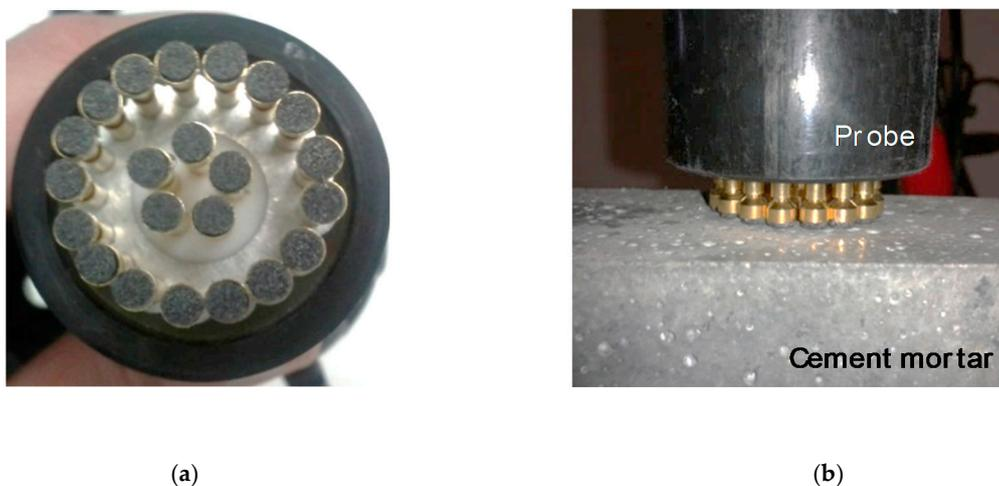
**Figure 5.** (a) Pin electrode arrangement in head of custom electrical probe and (b) Sample and probe during resistivity measurement.
